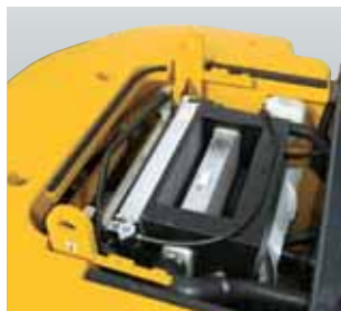
Locking engine hood provides protection while servicing
