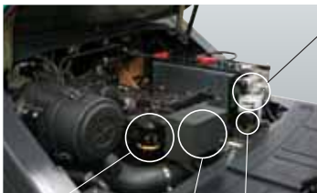
Relay and fuse boxes are conveniently located.
