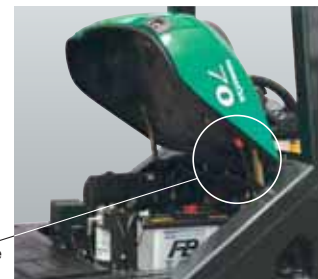
Locking engine hood provides protection while servicing
